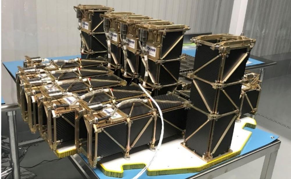
**Figure 19** Rocket Lab payload plate, payload configuration for NASA ELaNa-19 mission
