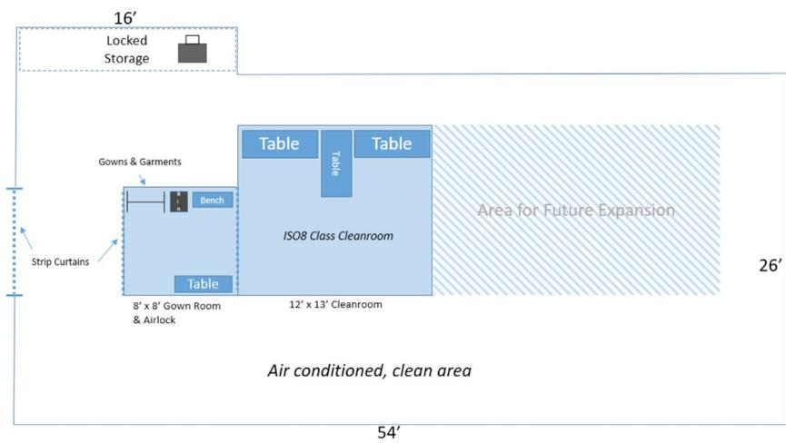
**Figure 47** Rocket Lab's Long Beach Payload Processing Facility Layout
