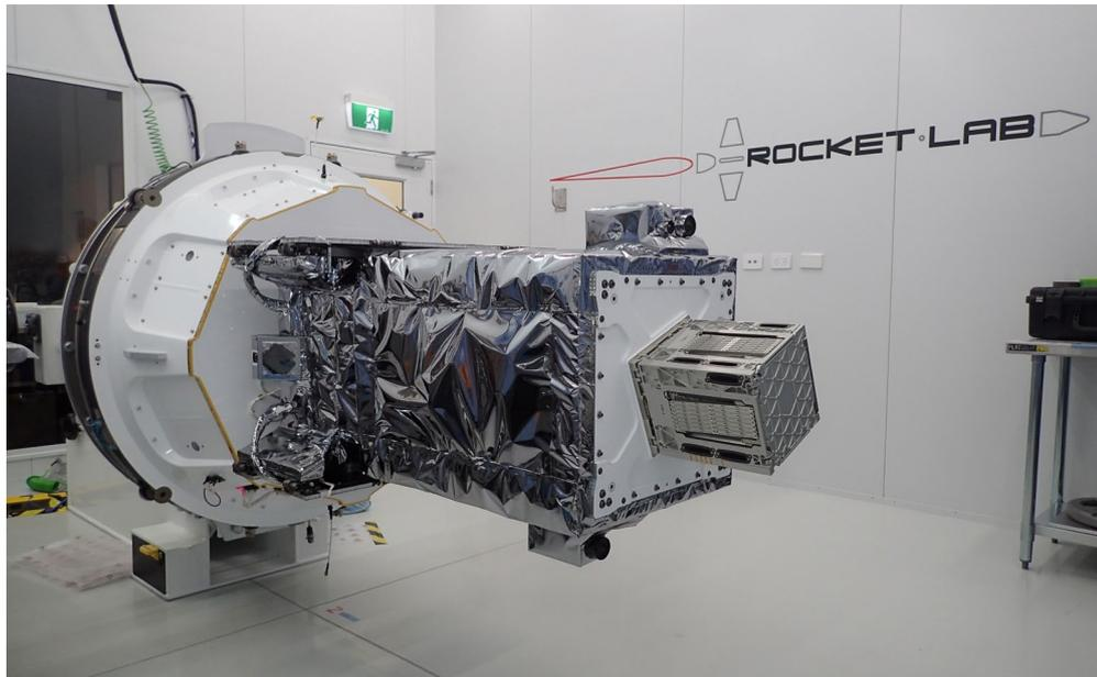
Figure 40 DARPA Spacecraft Intergrated with Rocket Lab's Kick Stage
