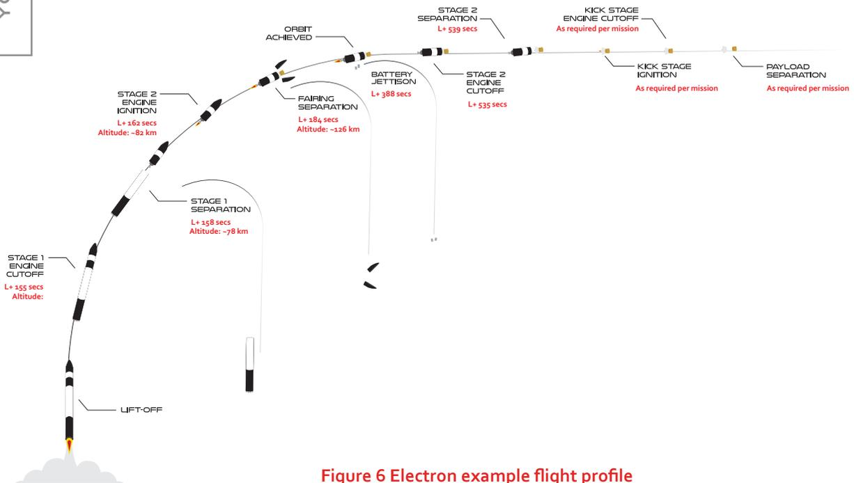
Figure 6 Electron example flight profile
