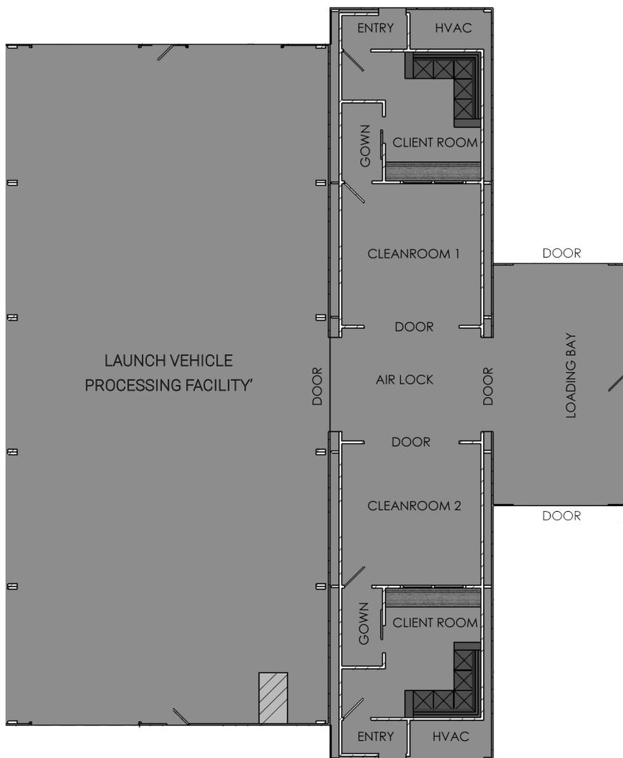
**Figure 44** The layout of the Payload Processing Facility at LC-1
