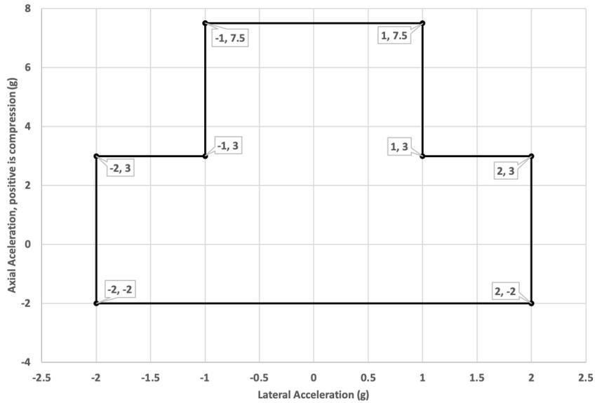
Figure 22 Electron Acceleration MPE
