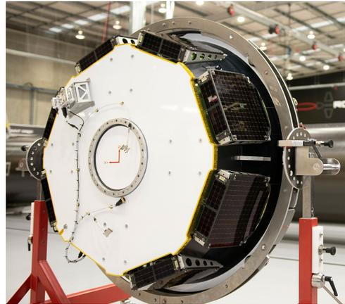
**Figure 10** Photon LEO configuration (payload plate view)
