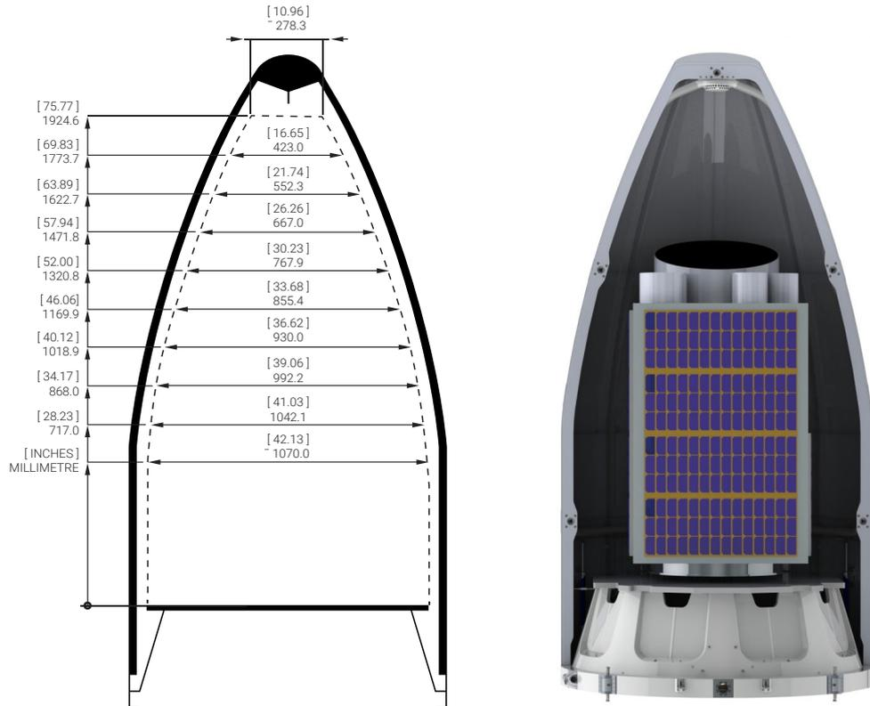
Figure 15 Fairing capacity & sample configuration inside of the fairing
