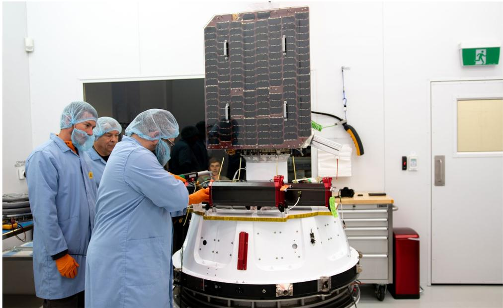
Figure 42 Flight 7 'Make It Rain' Payloads Intergrated With Rocket Lab's Kick Stage
