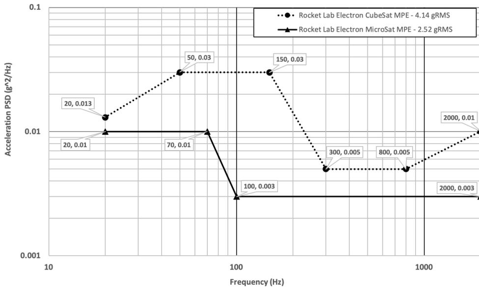
Figure 25 Electron Random Vibration MPE
