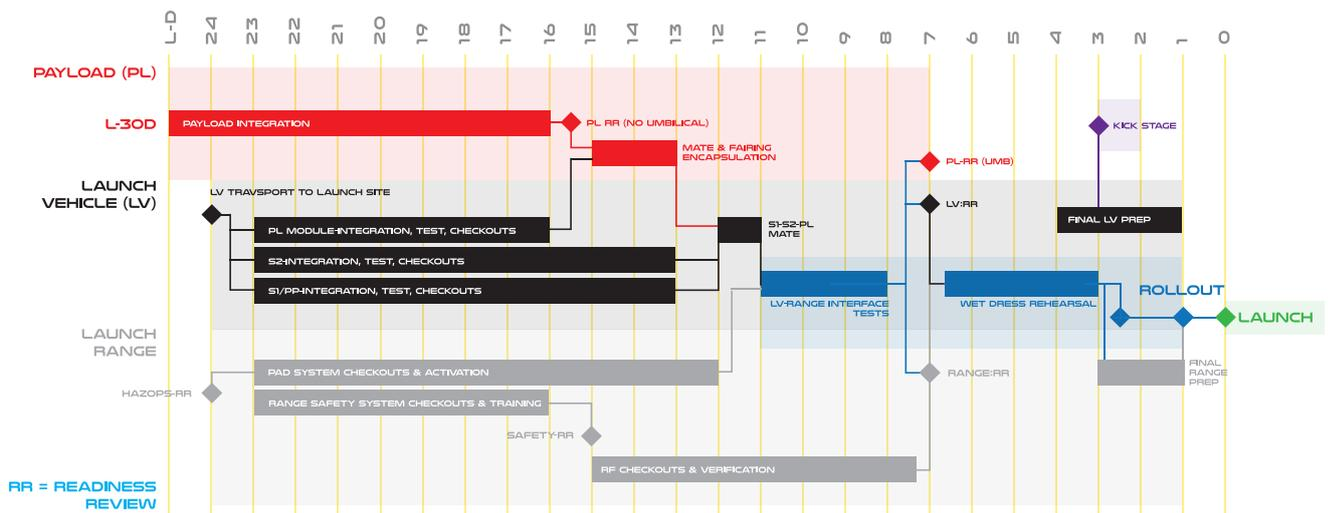
Figure 48 Example of a Standard Payload Processing Schedule
