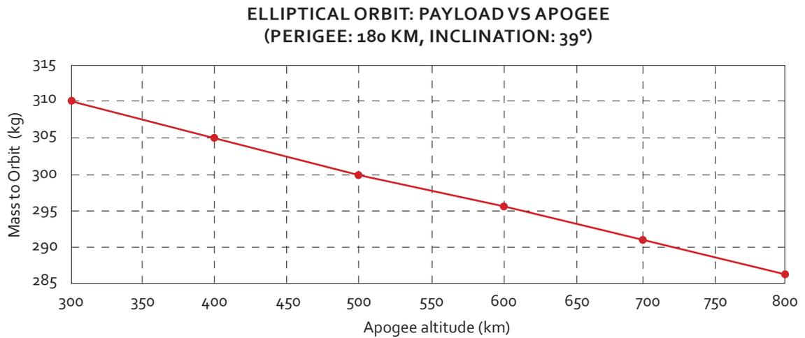
**Figure 13** Performance to a 180 km Perigee at 39° Inclination Elliptical Orbit
