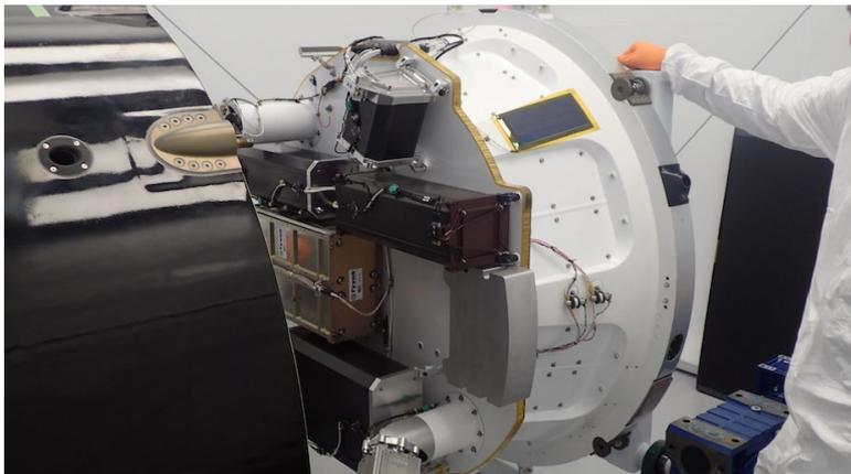
**Figure 7** Rocket Lab's Kick Stage being intergrated with the fairing
