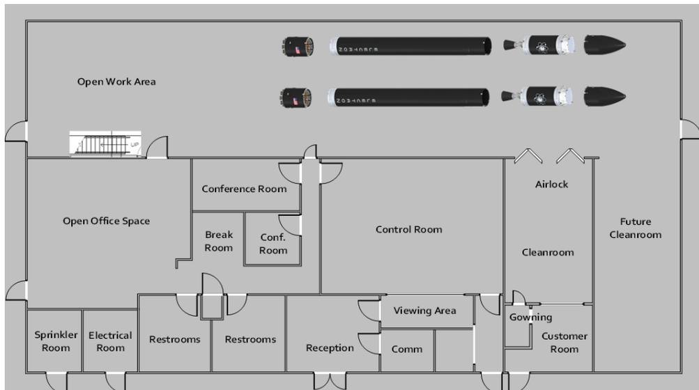
**Figure 46** The layout of the Payload Processing Facility at LC-2
