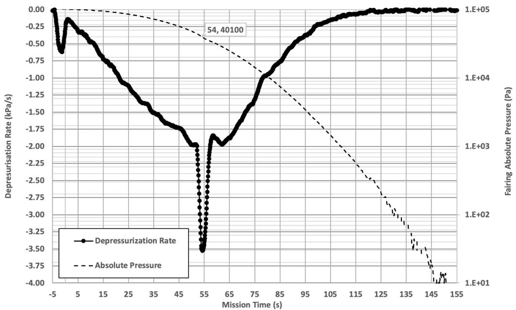
Figure 26 Electron Typical Fairing Venting Environment
